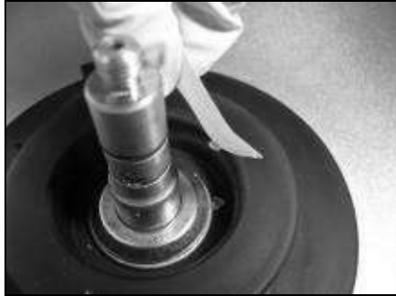
Removing plastic debris with tape.
